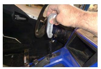
5. Slide the shifter handle body all the way onto the shifter lever.
