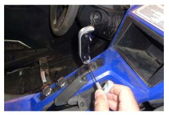
7. Install the left and right side plates (5) and (6) with the four flathead screws (2).
