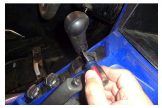
2. Remove the fastener from the right side of the shifter handle.
