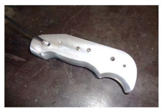
4. Thread the 4 small set screws (Item 4) about halfway into the shifter handle body (1) (two screws each side). Thread the large set screw (3) about halfway into the right side of the shifter handle body.
