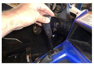
3. Pull the shifter handle off the shifter lever.
