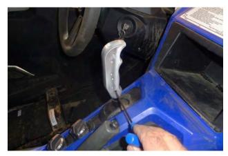
6. Tighten all five set screws to secure the shifter handle to the shifter lever.
