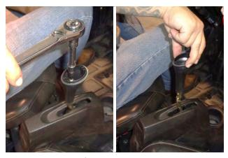
3. Remove the shifter handle screw, then pull the handle off the shifter lever.
