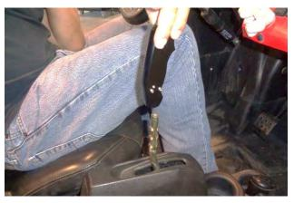
5. Slide the shifter handle body all the way onto the shifter lever.
