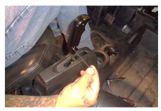
6. Tighten all 4 set screws to secure the shifter handle to the shifter lever.
