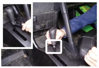
2. Turn off vehicle and chock tires, then carefully remove stock shifter handle.
