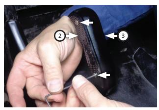
7. Install **left (2)** and **right (3) shifter plates** onto handle body using (x4) **screws (5)**.
