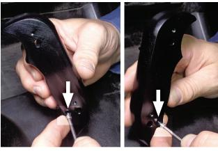
6. Install set screws onto handle body as shown.
