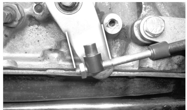
**31. Thread the swivel onto the cable** to about the middle of the threaded section, then reinstall (but do not yet tighten) the jam nut.
