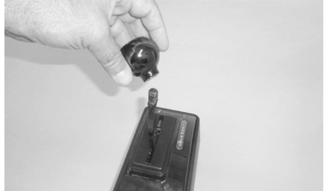
60. Apply **medium strength thread locker** to the shift lever threads. Carefully thread the **shift knob** all the way onto the lever and hand-tighten.
