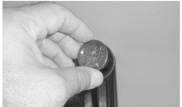
61. Align the **shift knob insert** as desired, and snap it into place.
