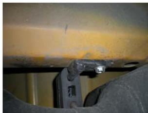
9) Place the **HA168** rubber hanger onto the hanger welded to the front of the muffler. Connect hanger assembly **#415HA** to the rubber mount and secure to the existing hole in the frame using the supplied 5/16” x 1” thread cutting bolt.
