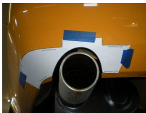
4) Because there is no cutout in the rear valance for the left side tailpipe, it will be necessary to make a new cutout. Follow the instructions on the attached template to properly align and make the cutout.
