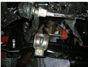
6) Place a supplied clamp onto the expanded end of over-axle pipe **#16739S** and slip it onto the back of pipe **#16738S**. Connect the hanger on the pipe to the rubber mount on the vehicle and tighten the clamp enough to hold, but still allow for adjustment. **Note:** On 2014 model vehicles, the rubber hanger mount that would accept the hanger on pipe **#16739S** has been omitted from the vehicle, therefore this hanger will not be used.
