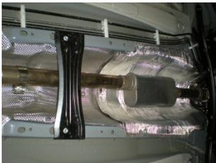
4) Using the 7/16" bolts, nuts and washers provided, bolt resonator assembly **15163S** to the back of the flex pipe flange. Be sure to replace the gasket. Support with a stand. Then reinstall the steel body brace removed in the previous step and tighten securely.
