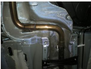
5) Place a supplied clamp onto the expanded end of pipe **#16738S** and slide onto the back of the resonator. Connect the hanger on the pipe to the rubber mount on the vehicle and tighten the clamp just enough to hold, but still allow for adjustment.
