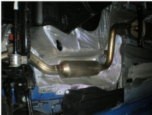
2) To remove the factory exhaust system you will have to cut the system in half. Cutting just behind the round resonator in the center of the system will allow both halves of the system to be removed easily. After cutting, support the rear muffler with a stand and remove the three hangers on this section from their rubber mounts. You can now lower this section from the vehicle. This section may take some turning and twisting to get the pipe over the rear axle.
