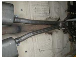
6) Slide a 2 1/2" clamp over each muffler inlet. Place Scavenger pipe assembly **#16789S** in its approximate position underneath the vehicle and connect the back of the Scavenger assembly into the muffler inlets and support with a stand. Tighten the clamps enough to hold, but still allow for adjustment.
