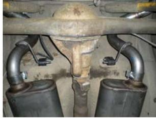
5) Place a provided 2 1/2" clamp onto the muffler outlets, then place the mufflers up into position and onto the front of the tailpipes. Slide the mufflers fully onto the tailpipes and support the mufflers with a stand. Tighten the clamps enough to hold, but still allow for adjustment. Be sure the rubber hangers are hanging vertically straight up and down.
