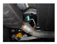
2) At the rear drivers' side of the vehicle, loosen the clamp on the muffler inlet. Support the muffler with a stand and remove the hanger at the rear of the muffler assembly from the rubber mount on the vehicle. Carefully lower the stand and remove the muffler from the vehicle.
