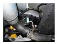
4) Place a provided clamp onto the inlet of muffler **#815430-298** and put up into position on the left side of the vehicle. Slide the inlet of the new Flowmaster muffler up to the tab on the factory pipe. Connect the hanger at the rear of the muffler assembly to the rubber mount on the vehicle and tighten the clamp at the inlet enough to hold, but still allow for adjustment.
