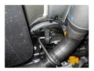
5) Place a provided clamp onto the inlet of muffler **#815430-299** and put up into position on the right side of the vehicle. Slide the pipes fully together and connect the two hangers on the muffler assembly to the rubber mounts on the vehicle. The two rubber mounts should hang vertically when the muffler is in the correct position. Tighten the clamp at the inlet enough to hold, but still allow for adjustment.
