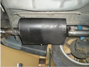
7) Place a provided clamp onto the inlet of muffler **#852460-290**. Connect the hanger on the body of the muffler to the rubber mount on the vehicle and then slide the inlet onto the back of over-axle pipe **#16835S**. Tighten the clamp on the muffler inlet enough to hold, but still allow for adjustment.
