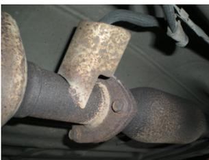
4) At the center of the vehicle, remove the three bolts attaching the factory mid pipe to the rear of the catalytic converter. Once the flange is loose, lower the pipe from the vehicle.
