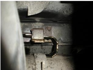
3) Support the rear muffler with a stand and slide the muffler assembly forward to release the hanger on the muffler from the rubber mount above the muffler. Then, slide the hanger just behind the rear axle from the rubber mount on the vehicle. Move the assembly toward the rear of the vehicle and remove.
