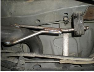
6) Place over-axle pipe **#16835S** into position over the rear axle and slide onto the back of inlet pipe **#16834S**. Connect the hanger on the pipe to the rubber mount on the vehicle and tighten the clamp enough to hold, but still allow for adjustment.
