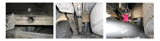
6) On the passenger side of the vehicle just forward of the rear tire, there is an oval hole in the bottom of the frame. Place the **467HA** under the hole with the round stock portion pointing to the inside of the vehicle. Use the **HA566** square plate as a backing plate on top of the frame and secure with the 3/8" bolt, nut and washers provided. Once secured, place a supplied HA168 rubber hanger onto the hanger mount as shown below.
