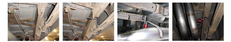
7) Place a supplied 4" clamp onto the inlet of muffler **#8540152-Z** and slide the muffler inlet fully onto the rear of pipe **#702TBS or 46168S.** Check to see that the muffler is level and tighten enough to hold, but still allow for adjustment.
