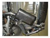
6) Place a provided clamp onto the inlet of muffler **#852559-317** and put up into position on the right outlet of the scavenger assembly. Slide the pipes fully together and connect the two hangers on the muffler assembly to the rubber mounts on the vehicle. Tighten the clamp at the inlet enough to hold, but still allow for adjustment. Repeat this step on the left side with muffler **#852559-316**.
