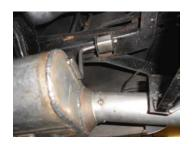
Place one of the supplied **HA602** rubber mounts onto the wire hanger of left muffler assembly **842458-342.** Place a provided clamp onto the muffler inlet, then place the assembly onto the back of the mid pipe and slide the two fully together. Support the muffler with a stand. Using a supplied 3/8" bolt, nut, washer and lock washer, bolt the HA602 hanger to the hole in the frame above the muffler outlet.
