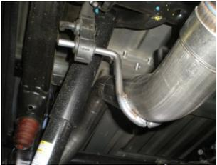
4) Slide a 3" clamp onto the muffler outlet neck. Place tailpipe #26410S into position over the axle and insert the hangers at the front and rear of the pipe into the rubber mounts on the vehicle and slide into the muffler outlet. Tighten the clamp just enough to hold, while still allowing for adjustment.
