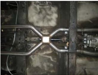
1) After installing either the **81094** or **81096** downpipe kits, place a provided 2.25" clamp onto the expanded ends of X-pipe assembly **86200S**, then slide onto the back of the manifold pipes, be sure that the pipes are fully slid together. Place a stand under the rear of the assembly and tighten the clamps enough to hold, but still allow for adjustment. The Flowmaster embossing will be toward the ground.
