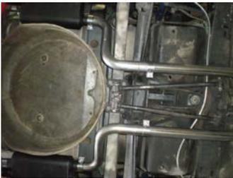
2) Place a provided clamp onto both outlets of X-pipe assembly **86200S**. Place the expanded end of mid pipe **86205S** onto the right outlet of the X-pipe assembly. Rotate the pipe up into position and support the rear of the pipe with a stand. Tighten the clamp enough to hold, but still allow for adjustment. Repeat this step on the left side of the vehicle with pipe **86204S**.
