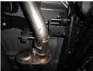
6) Place a provided 3" clamp onto the muffler outlet, place the over-axle pipe **#26478S** into position over the axle and slip into the muffler outlet. Connect the hangers on the pipe to the rubber mounts on the vehicle. Tighten the clamp just enough to hold in position.
