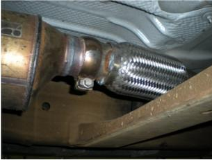
4) Place inlet pipe assembly **#26477S** into position onto the ball connection behind the catalytic converter. Connect the hanger on the pipe to the rubber mount on the vehicle, then reinstall the clamp onto the ball connection and tighten enough to hold but still allow for a small amount of adjustment.
