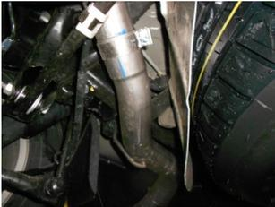
7) Place a provided 3" clamp onto the expanded end of exit pipe **#26479S** and slide onto the back of the over-axle pipe. Be sure the two pipes slip completely together and connect the hanger on the pipe to the rubber mount on the vehicle. Tighten the clamp just enough to hold in position.
