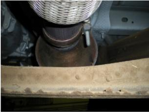
3) Using a 15mm wrench, loosen the bolt on the clamped ball connection behind the catalytic converter. Separate the three wire hangers from the rubber mounts on the vehicle and lower the inlet pipe and muffler from the vehicle.
