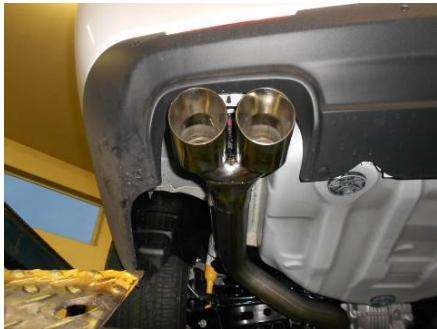
3) Place a supplied clamp onto the left muffler outlet. Place the left tailpipe **#26530S** into position and starting from the rear, connect the hangers on the tailpipe to the rubber mounts on the vehicle. Slide the tailpipe fully into the muffler outlet. Adjust the tailpipe so that the stainless tip is level and centered in the bumper cut-out. Tighten clamp enough to hold, but still allow for adjustment. Repeat this step for right tailpipe **#26531S**.
