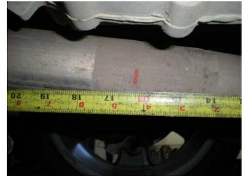
2) Begin by measuring back 16 1/4" from the edge of both factory mufflers and make a mark on the pipes (see photos above). Once you have double checked that the measurements are correct, cut both pipes through at the marks. Remove the two hangers on each tailpipe assembly from the rubber mounts on the vehicle and remove the tailpipe assemblies from the vehicle. Carefully deburr the end of the pipes with a file or die grinder.
