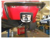
Place one of the supplied **HA602** rubber mounts onto the wire hanger of left muffler assembly **842555-354**. Place a provided clamp onto the muffler inlet, then place the assembly onto the back of the mid pipe and slide the two fully together. Support the muffler with a stand. Using a supplied 3/8" bolt, nut, washer and lock washer, bolt the **HA602** hanger to the hole in the frame above the muffler outlet.
