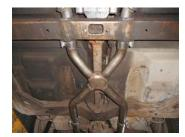
1) After installing either the **81101** or **81103** downpipe kits, place a provided 2.25" clamp onto the expanded ends of X-pipe assembly **86233S**, then slide onto the back of the manifold pipes, be sure that the pipes are fully slid together. Place a stand under the rear of the assembly and tighten the clamps enough to hold, but still allow for adjustment.
