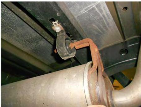
2) Begin by applying a lubricant to each of the rubber exhaust isolators as well as the two front flange bolts. This will make the removal and installation process much easier.
