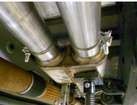
5) Install a provided clamp onto each of the muffler outlets. Then place the right side tailpipe **#26533S** into position over the axle and into the right side muffler outlet while also connecting the hanger on the pipe to the rubber mount on the vehicle. Tighten the band clamp enough to hold, but still allow for adjustment.
