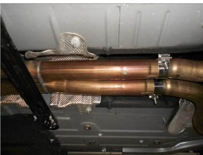
2) Begin by placing a supplied 2 ¼" clamp onto each of the slip fits on Scavenger pipe **#86331S**. Place the Scavenger pipe onto the back of the stock head pipes (make sure the Flowmaster embossing is facing the ground). Level and center the assembly in the drive line tunnel and support with a stand. Tighten the two clamps enough to hold, but still allow for adjustment. Reinstall the two body braces onto the vehicle and tighten securely.
