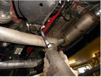
2) Begin by measuring back 1 ½" from the rear of the suspension cross-member shown in the photos above and make a mark on both pipes. Support the exhaust system both in front and behind the area to be cut, then once you've double checked that the measurements are correct, cut both pipes at the marks. **Note: Use caution when cutting!**
