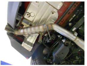
3) Adjust and level the two muffler assemblies to provide a satisfactory fit. They can also be adjusted forward or back to get the desired position in the rear bumper cut-outs. A minimum of 1/2" clearance around all parts of the system must be maintained; while keeping suspension travel and vibration in mind. After adjustments have been made, and you are satisfied with the fit, you may now securely tighten the two muffler inlet clamps.
