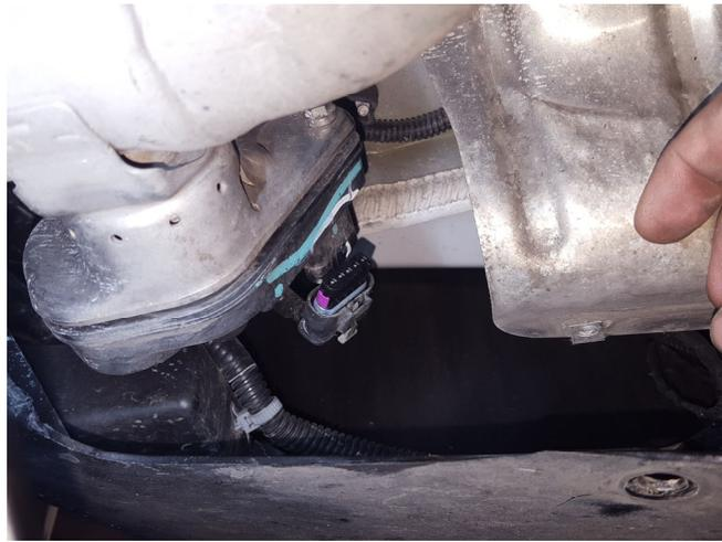
3) Behind each rear tire, remove screws (x2 ea.) attaching lower cover to frame. Unplug electrical connection from actuators then dismount both front wire hangers on muffler from rubber isolators.
