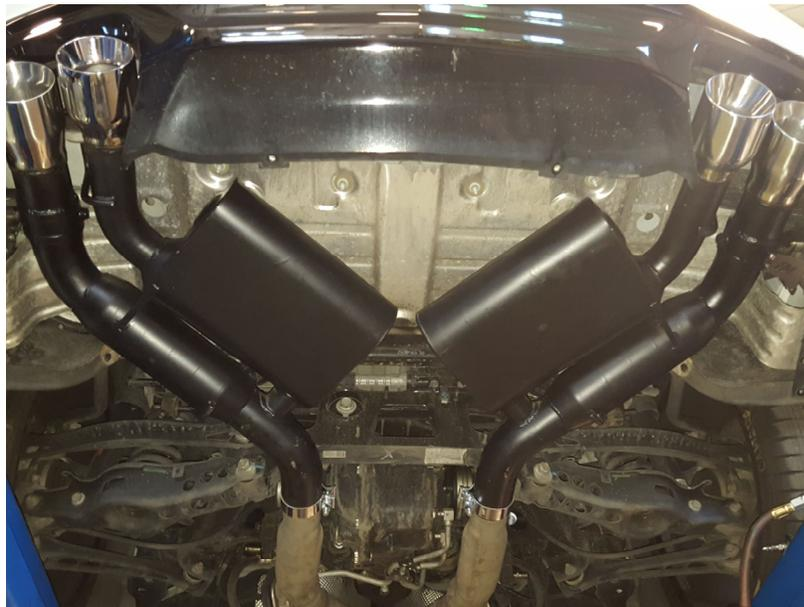
3) Adjust and level muffler assemblies to provide a satisfactory fit. They can also be adjusted forward or back to get desired position in rear cut-outs. Maintain a minimum of 1/2" clearance around all components; keeping suspension travel and vibration in mind. After adjustments have been made to your satisfaction, securely tighten both muffler inlet clamps.
