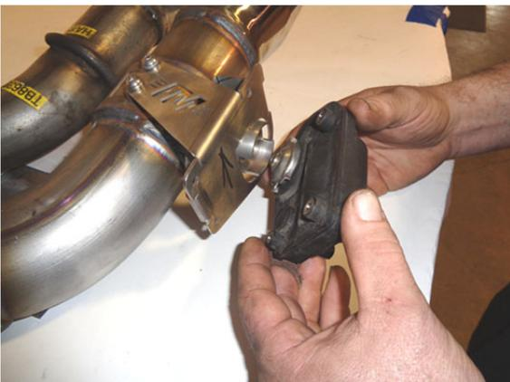
1) Remove bolts (x3) securing exhaust actuators to factory muffler assembly. Place them onto mounts on new Flowmaster units then fasten them by re-using bolts (x3).
