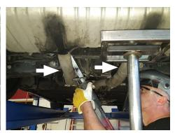
4. Remove screws (x4) attaching lower cover to frame to Mark factory driver and passenger tailpipes, 1" in front of bend as indicated.
