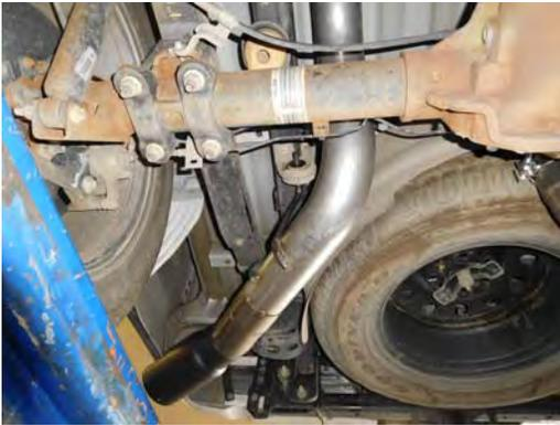
4) Install a provided clamp onto the muffler outlet. Then place tailpipe **#46197S** into position over the axle and into the muffler outlet while also connecting the hangers on the pipe to the rubber mounts on the vehicle. Tighten the band clamp enough to hold, but still allow for adjustment.
