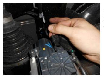
6) Reconnect the two electrical plugs removed in step 2 of the removal instructions back onto the tailpipe actuators now installed on the new Flowmaster tailpipes.
