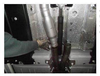
4) Place a supplied 3" clamp onto the inlet neck of both mufflers. Slide the mufflers onto the back of the Scavenger pipe assembly about 1-3/4" and support with stands. Level the mufflers and tighten the clamps enough to hold, but still allow for adjustment.
