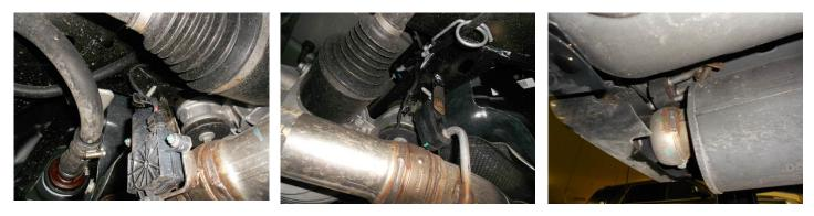
3) Once the factory system is out of the vehicle, use a 5/16 wrench to remove the three nuts securing the actuator to the mounts on the tailpipes. Remove the actuator and spring from the mount on each tailpipe.
