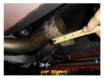
3) Begin the installation by placing a supplied 2-1/2" clamp onto each of the inlets of the Scavenger pipe **#26640S.** Then place the Scavenger pipe onto the back of the stock head pipes (the offset outlet pipe should be oriented to the passenger side). Level and center the assembly in the drive line tunnel and support with a stand. Scavenger pipe should slide over factory head pipe about 2". Tighten the two clamps enough to hold, but still allow for adjustment.
