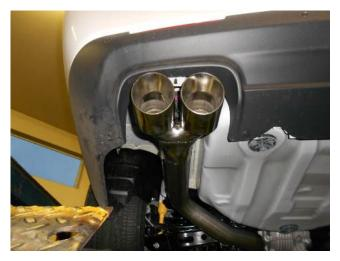
5) Place a supplied clamp onto the left muffler outlet. Place the left tailpipe **#26628S** into position and starting from the rear, connect the hangers on the tailpipe to the rubber mounts on the vehicle. Slide the tailpipe fully into the muffler outlet and adjust the tailpipe so that the stainless tip is level and centered in the bumper cut-out. Tighten clamp enough to hold, but still allow for adjustment. Repeat this step for right tailpipe **#26626S**.
