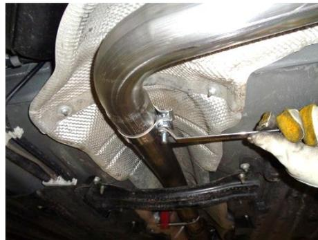
6) Place a supplied clamp onto the back of muffler assembly **815425-476**. Then place intermediate pipe **#86447S** into position from the front of the rear axle, and slip it onto the back of the muffler. Support the rear of the pipe with a stand if necessary and tighten the clamp enough to hold, but still allow for adjustment.
