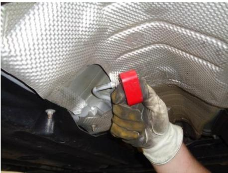
4) Place the provided **HA1640** polyurethane hangers onto each of the four factory hanger mounts on the vehicle.
