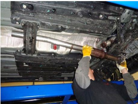
5) Using the nuts removed in step 3 above, bolt muffler assembly **815425-476** to the back of the flex pipe flange. Be sure to replace the gasket. Connect the hangers on the assembly to the rubber mounts on the vehicle and tighten the flanged connection securely. Re-install the steel body brace removed in the previous step and tighten securely.
