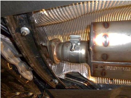
5) Place a supplied clamp onto the inlet of muffler **#15191S**, slide the muffler onto 873TBS completely and support the muffler with a stand, tighten the clamp enough to hold but still allow for adjustment.
