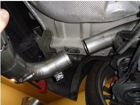
9) Place a supplied clamp onto the front of the exit pipe assembly. Slide the exit pipe assembly over the back of the over-axle pipe and connect the right hanger on the assembly to the rubber mount on the vehicle. Using the factory bolts, reinstall the left hanger back onto the frame of the vehicle. Tighten the clamp enough to hold, but still allow for adjustment.
