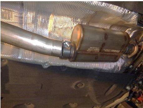
6) Place a supplied clamp onto the outlet of muffler **#15191S**, slide intermediate pipe **#26684** into the back of the muffler and connect the hanger on the pipe to the rubber mount on the vehicle. Support the pipe with a stand and tighten the clamp enough to hold, but still allow for adjustment. Then reinstall the steel body brace removed in step 3 above and tighten securely.
