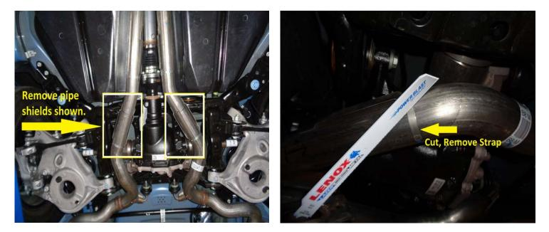
3) Begin by removing the two pipe heatshields indicated in the first picture above. Cut thru the strap at the rear of the shield, then lift and lower the shield a few times to break the weld at the front of the shield. Remove.
