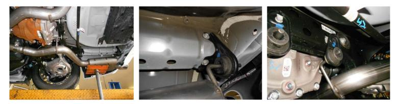
2) Place the right muffler assembly **#8430412-483** up into position and slide onto the factory pipe approximately 2-1/2". Support the assembly with a stand and remount the rear hanger mount to the frame and tighten securely. Remount the front hanger to the cross member and tighten securely. Leave the clamp on the inlet loose for now. Repeat this step with muffler assembly **#8430412-484** on the left side of the vehicle.
