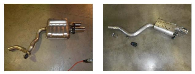
1) Place the new Flowmaster muffler units next to the factory units and swap the front and rear hanger mounts from the stock mufflers to the Flowmaster assemblies. Also, place a provided 2-1/2" clamp onto the inlet of each assembly. Tighten the clamp just enough to hold in place.
