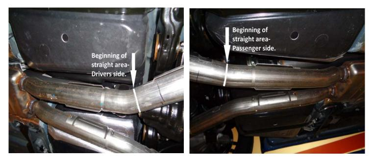
4) Behind the factory center resonator, follow the pipes back just past the second bend of each pipe, make a mark on each pipe where the bend ends and the straight area begins. See above photos.
