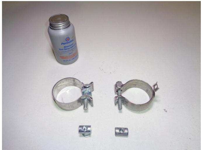
9. Transfer hangers from factory muffler assembly to **left (2) and right (1) muffler assemblies**. Place **clamp (3)** onto muffler inlets.
