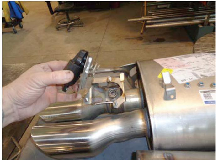
12. Install actuator onto new valve by lining spring arm to notch in valve shaft, then lower it into place. The holes in actuator assembly should line up with holes in mount, rotate if required. Complete this step on both valves.
