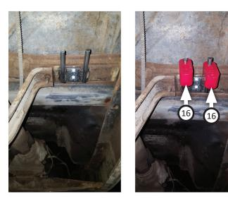
10. Hang **h-pipe assembly (3)** in front frame hanger as shown.
