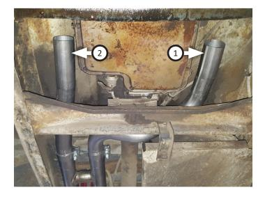
**NOTE:** This kit includes **rear (8-9)**, **side (7)** and **dump (10-11)** exit pipes. The exit pipes are left long in order to let you decide how your exhaust should look. Choose which style you would prefer, then use corresponding parts to complete this step.
