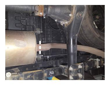
4. Support muffler and disassemble wire hangers from isolators. Remove and retain (x2) bolts from flange then disconnect and remove muffler section from vehicle.
