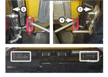
Connect muffler (1) to mid pipe, inserting wire hanger into rubber hanger. Adjust exhaust components for fit; maintaining 1/2" clearance and compensating for suspension, travel and vibration then tighten all clamps.
