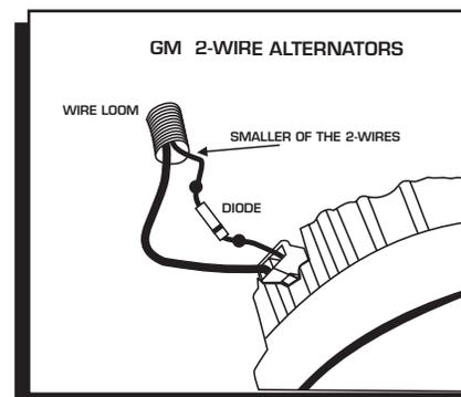
Figure 9 Installing the Diode to a 1973-1983 GM Vehicle.
