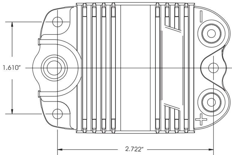
Figure 5 Mounting Template.
