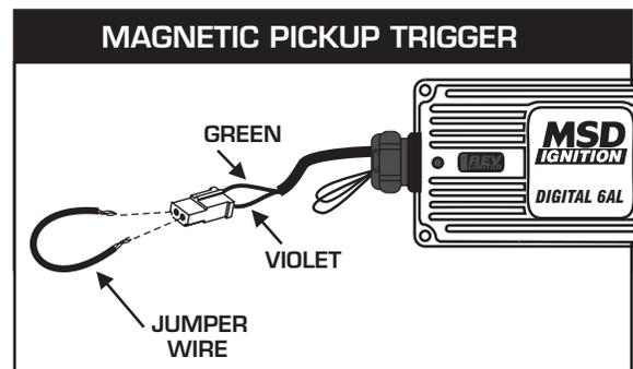
**Figure 11 Checking for Spark with the Mag Pickup.**
