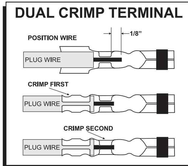
Figure 12 Crimping a Dual Crimp Terminal.
