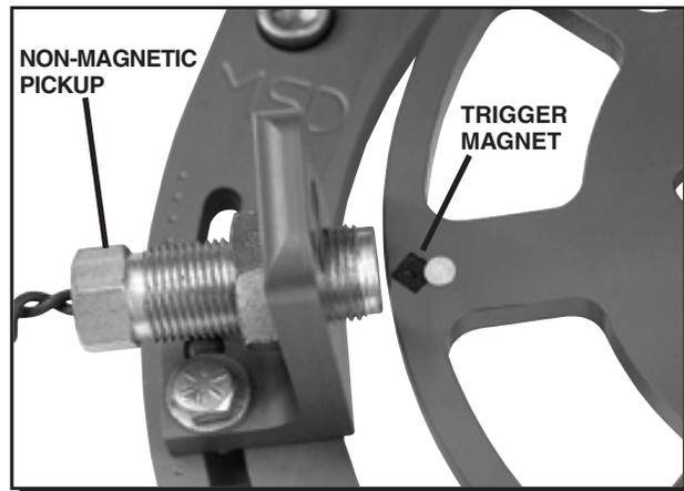
Figure 2 - MSD Flying Magnet Crank Trigger.
