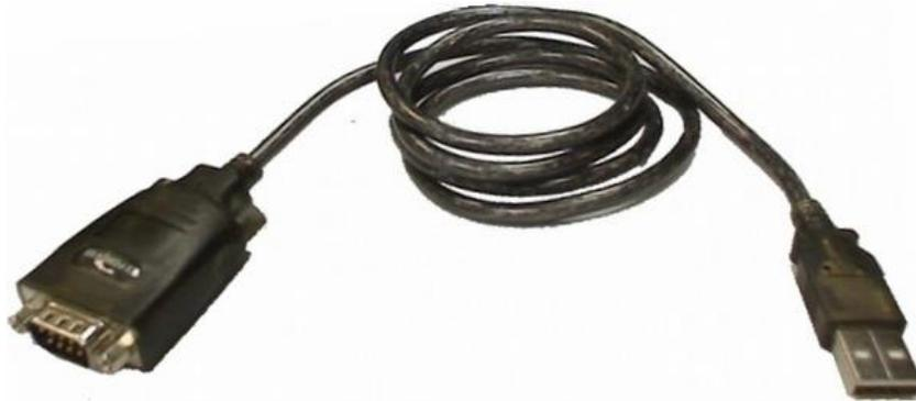
**Please note: You must install the DataLink II CD provided before plugging in your USB to Serial adapter**
