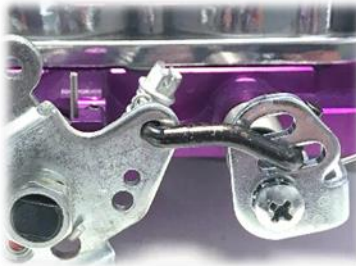
Super Progressive Link, Black Top hole, lower slot. 60% primary before secondary opens.
