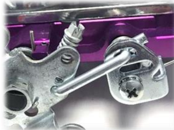
1 to 1 Link, Silver Third hole down, top slot Primary and secondary open at same time.
