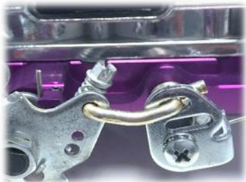
Medium Progressive Link, Gold Top hole, top slot. 40% primary before secondary opens. This is standard linkage for most applications.
