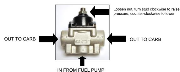
Installation of this regulator should follow the above illustration to route the fuel lines. The ports are 3/8" pipe thread. Use the provided mounting bracket to mount the regulator.
