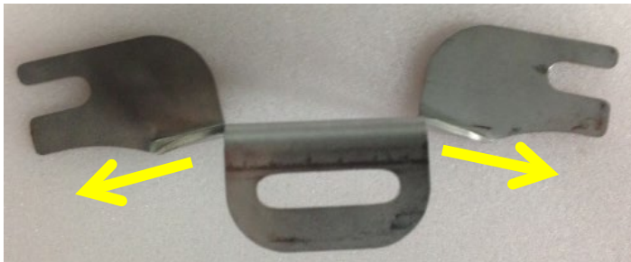
MTBRGMK – After Bending ( Bend at thin sections )
