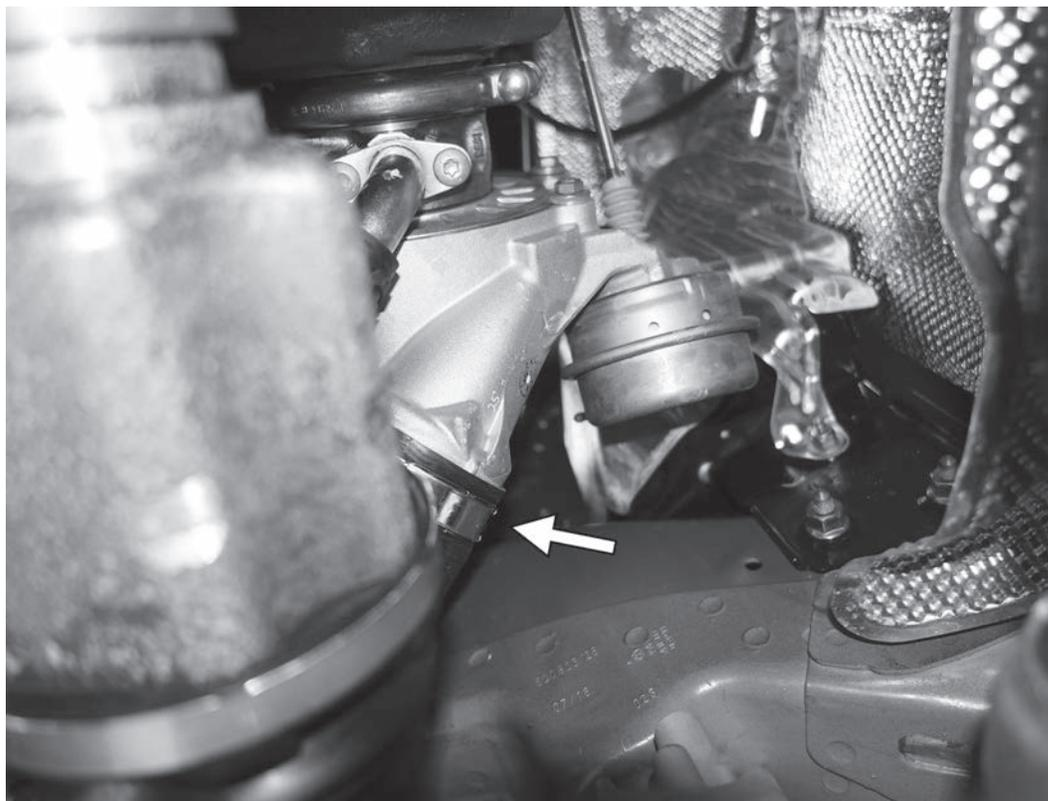
15) Loosen the clamp on the turbocharger outlet hose, nearest the turbocharger. A flathead screwdriver or 7mm socket will work for this. The clamp is affixed to the hose, so only loosen the clamp.
