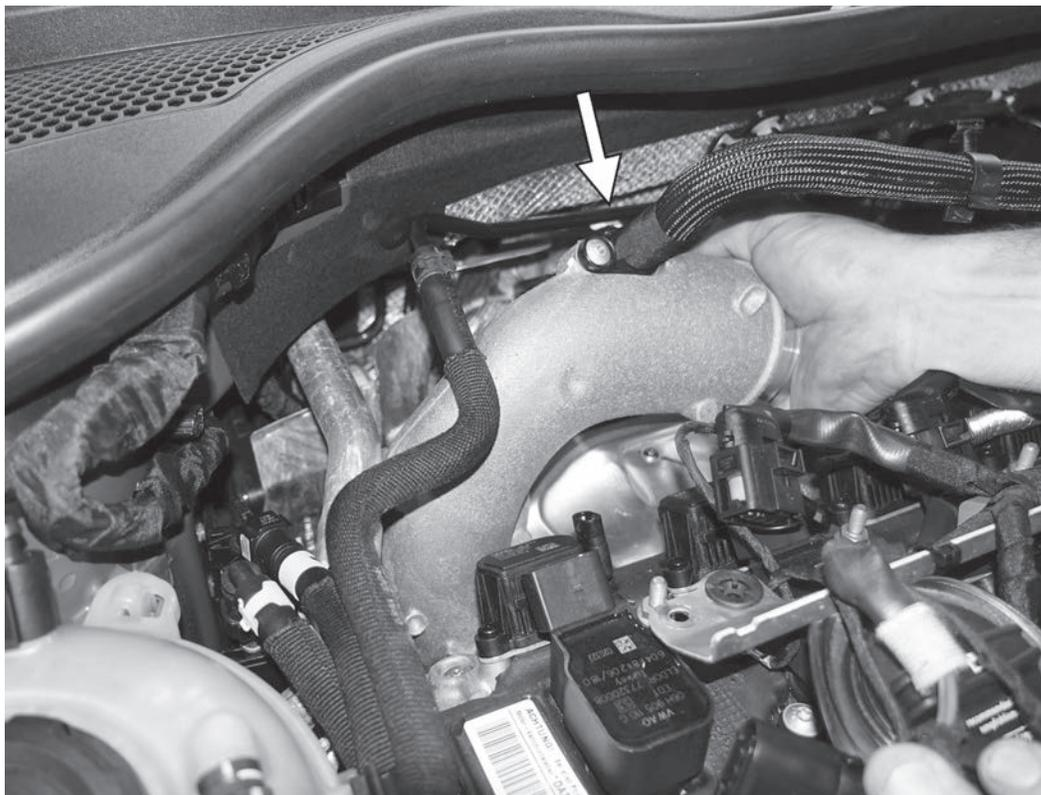
21) Lift and remove the stock turbo inlet pipe from the car, along with the attached PCV hose.
