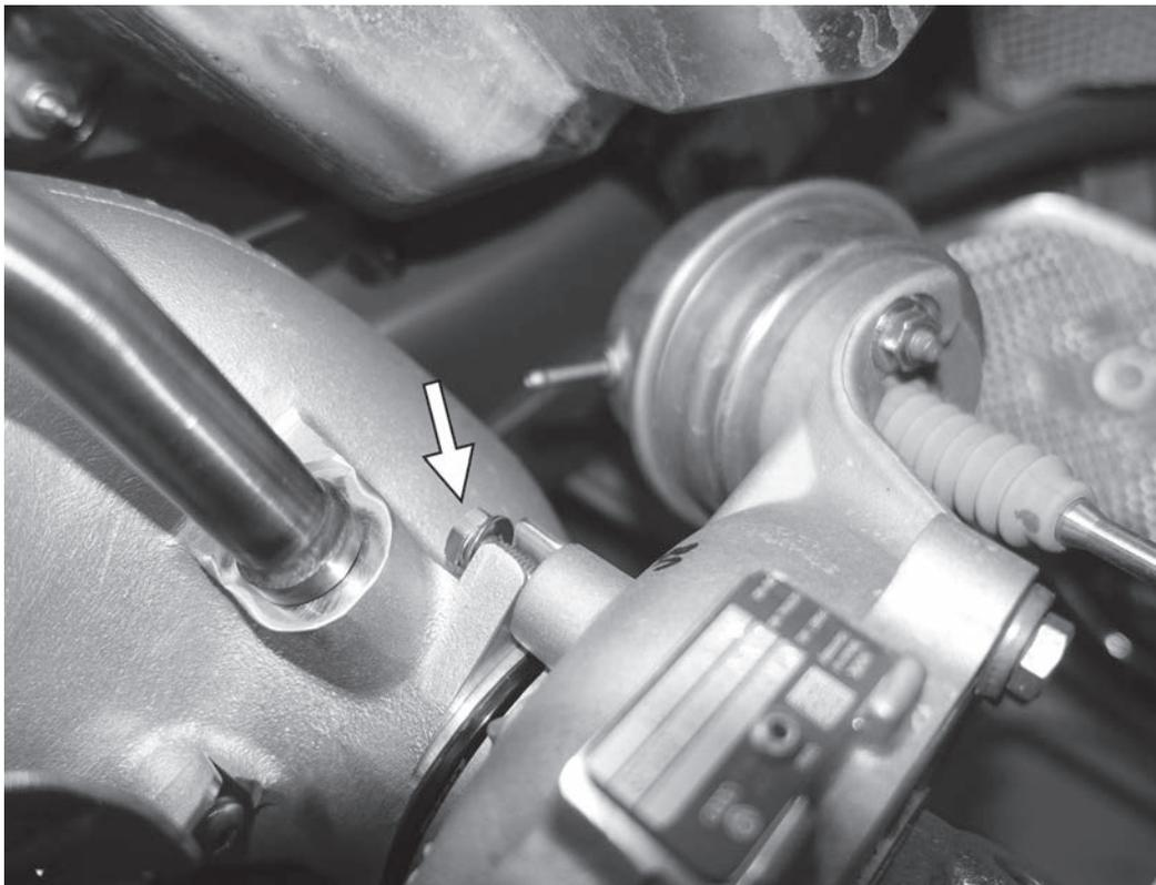
27) On the supplied 10mm screw, put a drop of medium strength, blue threadlocker, like Loctite 246. Install the wedge lock washer onto the screw, being careful not to separate the two halves of the lock washer. Very loosely install the supplied 10mm screw and wedge lock washer into the upper mounting hole on the turbo, holding the APR turbo inlet pipe to the turbocharger.
