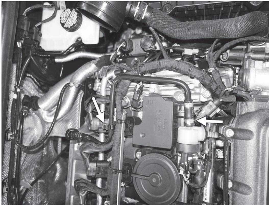
3) Cut the ear clamp on the rubber hose at the crankcase solenoid valve (N546) and separate the hose from the valve. Remove the clip on the back side of the plastic hose and remove the hose from the car.
