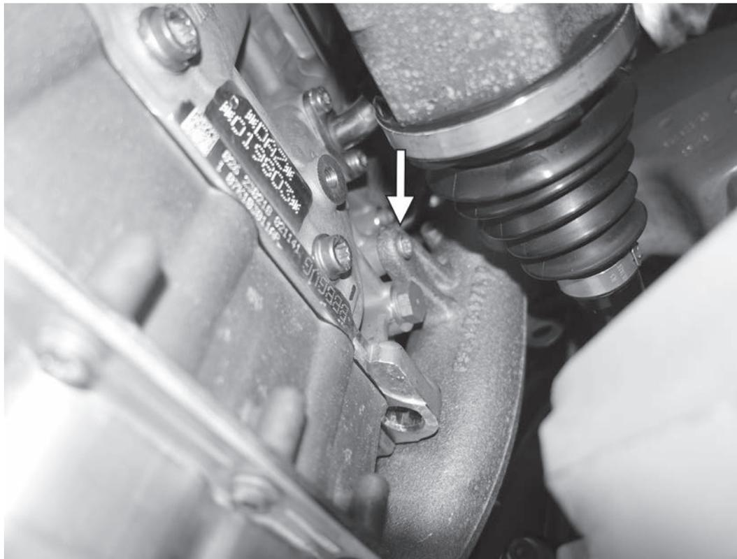
17) Remove the 10mm triple square screw holding the turbo outlet pipe to the back of the engine block.
