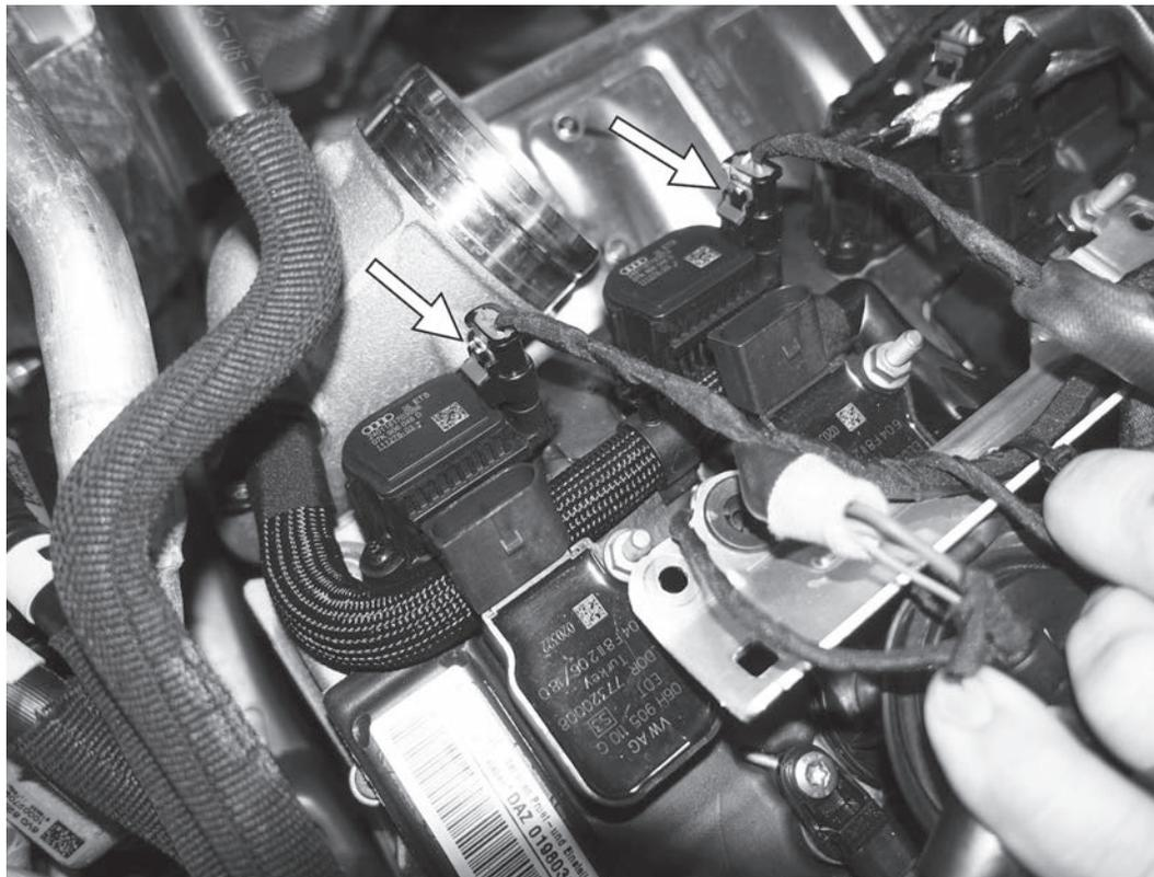
9) Disconnect the electrical connectors to the two exhaust valvelift solenoids, just under the ignition coil connectors.
