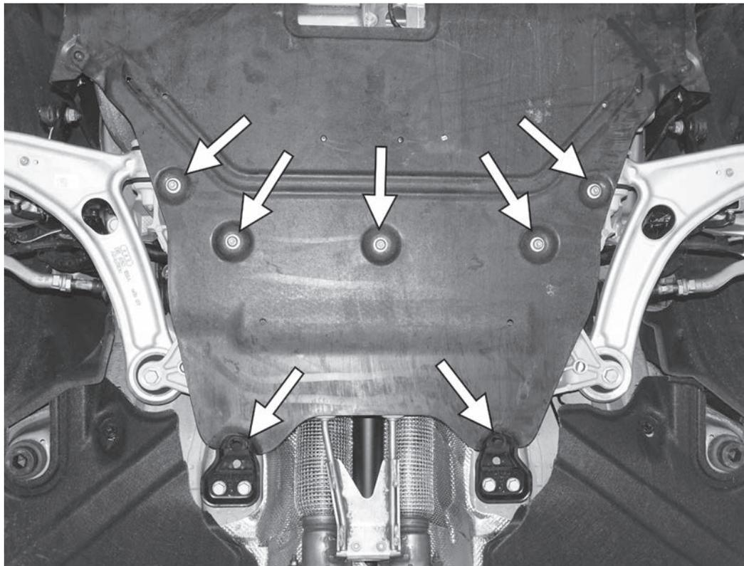
13) Remove the two push pin style connectors from the back of the belly pan. With an assistant holding the belly pan, remove the five T45 screws in the middle of the belly pan, and remove the it from the car.
