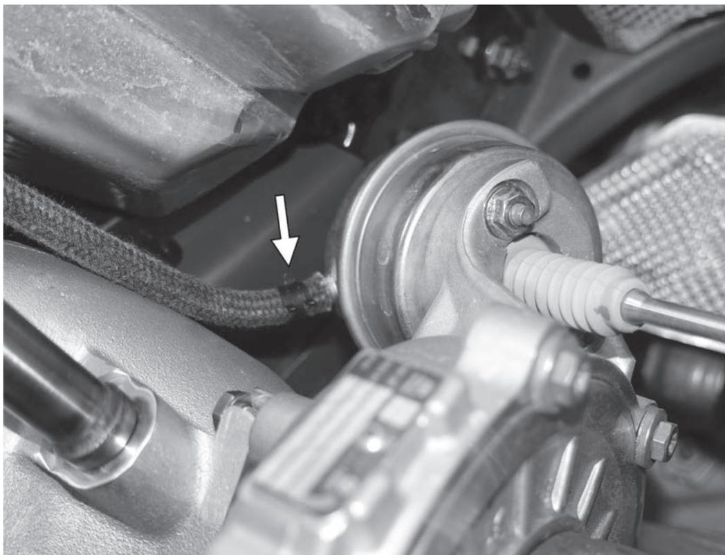
41) Connect one end of the braided hose to the port on the turbocharger wastegate. Route the rest of the line up, following the right side of the APR turbo inlet pipe.
