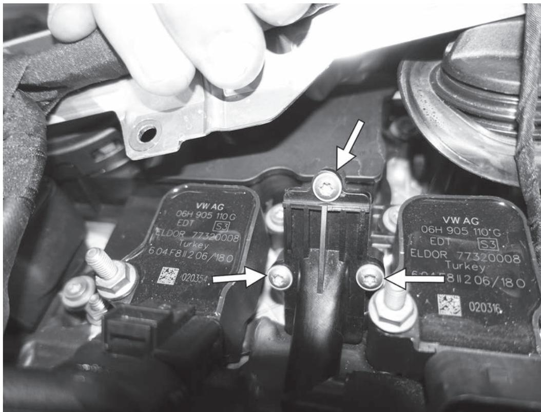
37) Reroute the PCV hose as it was originally from the factory, and reconnect it to the PCV valve between ignition coils #1 and #2 with the three original T20 screws. Torque the screws to 31 in-lbs (3.5Nm).
