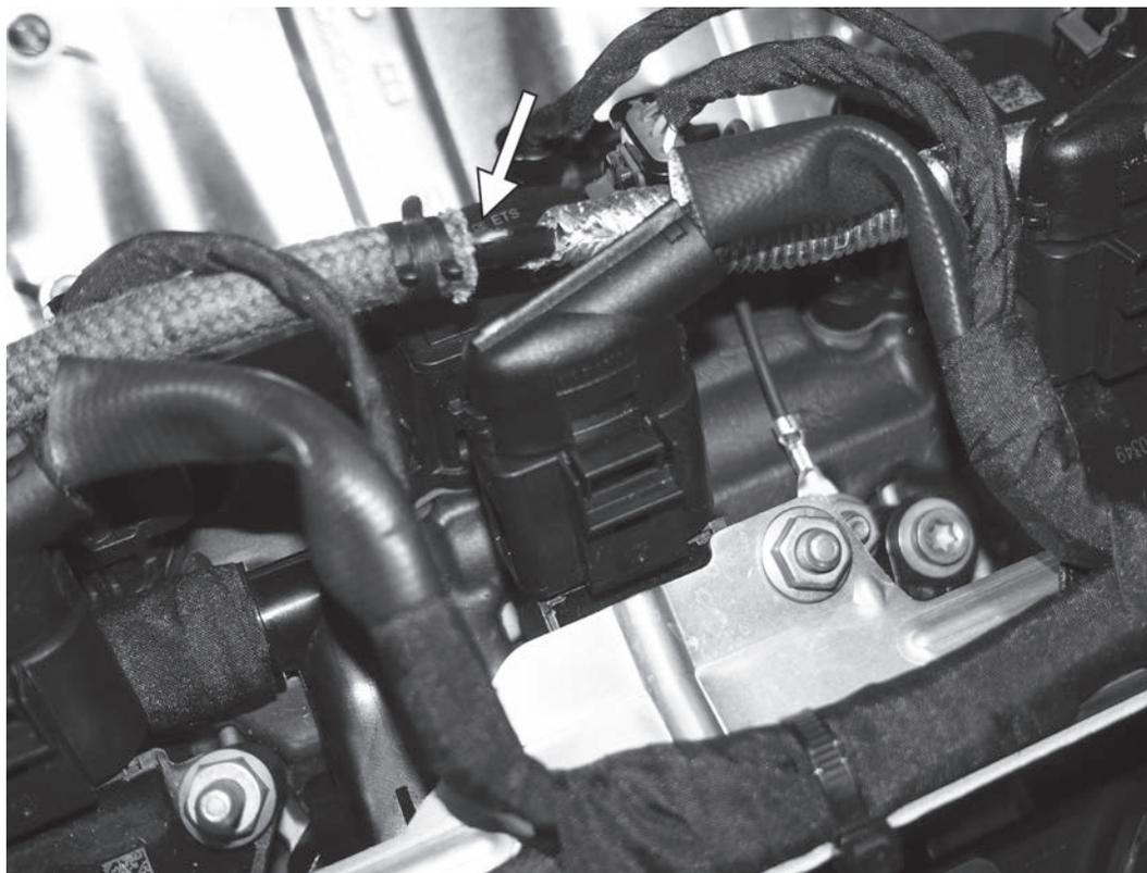
43) Connect the other end of the braided line to the plastic hose that goes to the boost control valve (N75). Secure the connection with the crimp clamp.
