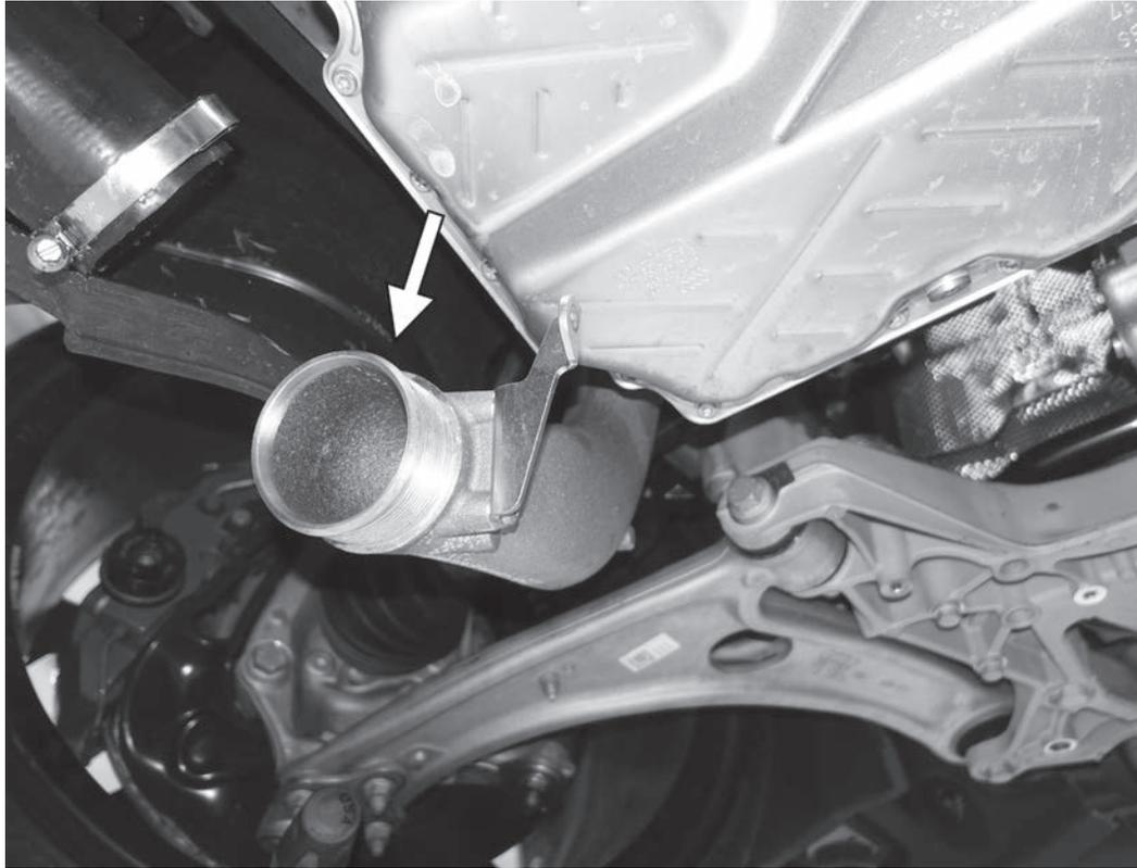
19) Remove the turbo outlet pipe by pulling the pipe down from the car. It may be necessary to use a large, angled pick to separate the rubber hose from the turbocharger outlet at the previously loosened clamp.
