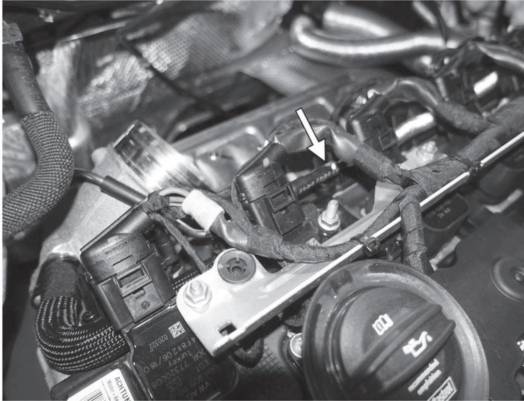
5) Follow this hard line up until it goes to a rubber line, and then back to a hard plastic line, roughly behind the cylinder #3 ignition coil. Disconnect the rubber hose from the plastic line and remove the entire hose assembly from that point to where it attaches to the wastegate, on the back of the turbocharger.
