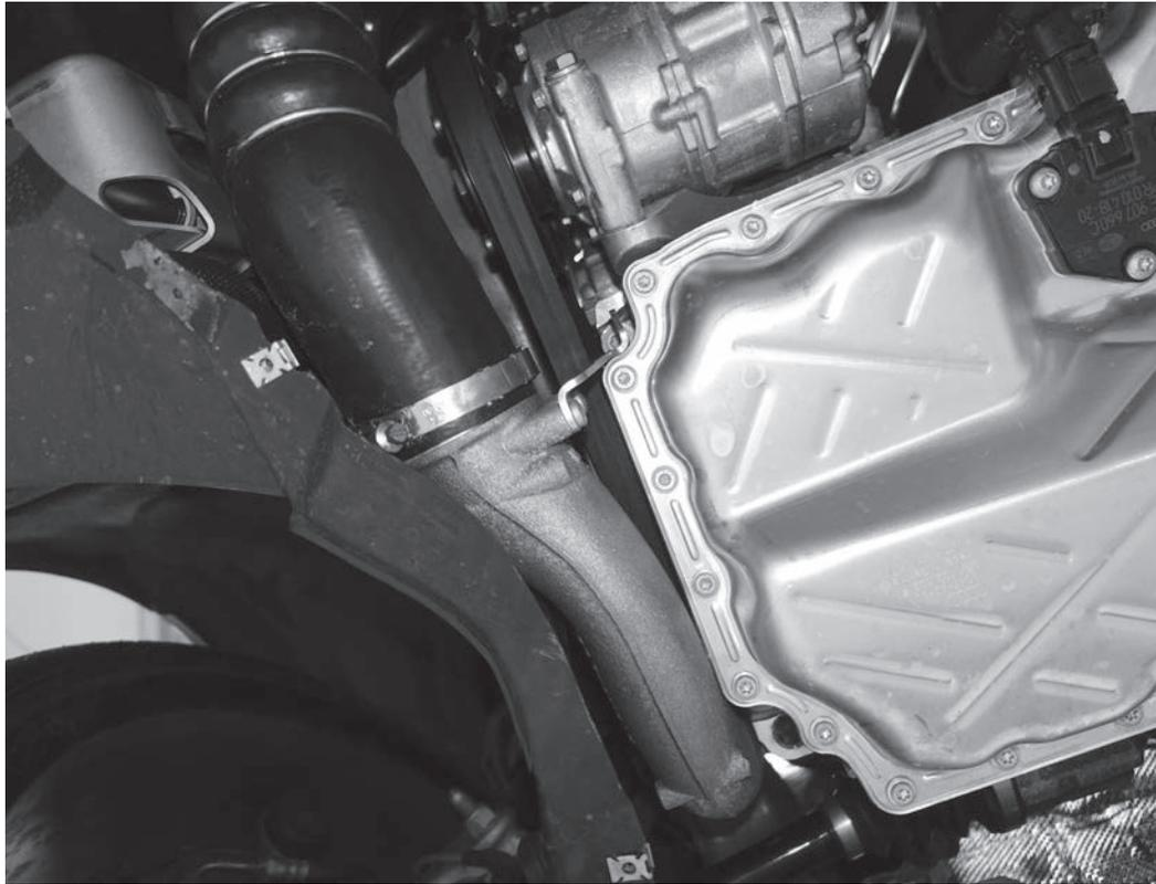
29) Reinstall the stock turbo outlet pipe, connecting the hose from the pipe to the turbocharger outlet and connecting the intercooler hose to the front side of the pipe. Loosely reinstall the T30 screw holding the front outlet pipe bracket to the engine block.
