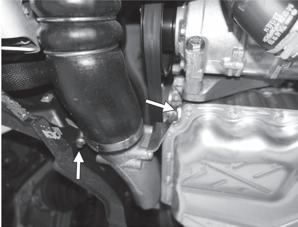
31) Torque the T30 screw on the turbo outlet pipe bracket to 70 in-lb (8Nm). Tighten the 7mm screw on the hose clamp connecting the outlet pipe to the intercooler hose by torquing it to 48 in-lb (5.5Nm). Do not overtorque the clamp or the screws.
