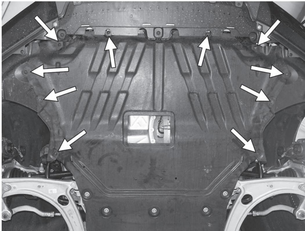
33) With an assistant, raise the belly pan back onto the car. Install the ten T25 screws on the front of the belly pan.
