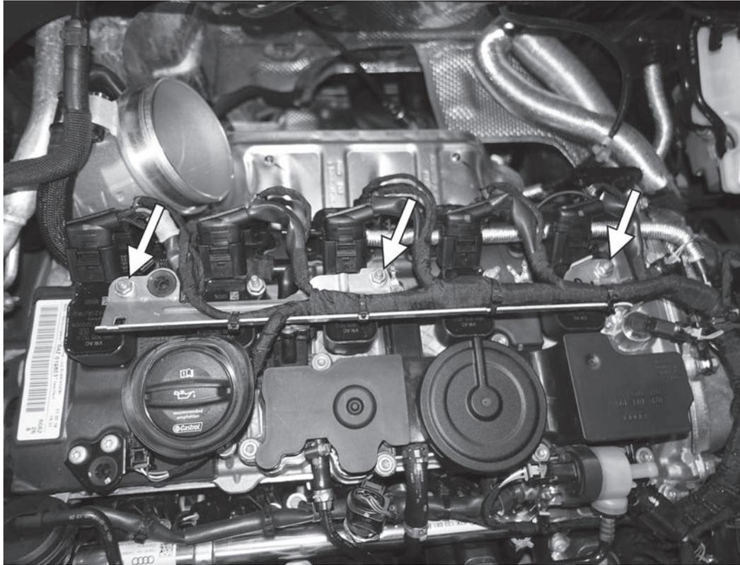
39) Install the three 10mm nuts that hold the metal bracket to the ignition coils, and torque to 62 in-lbs (7Nm).
