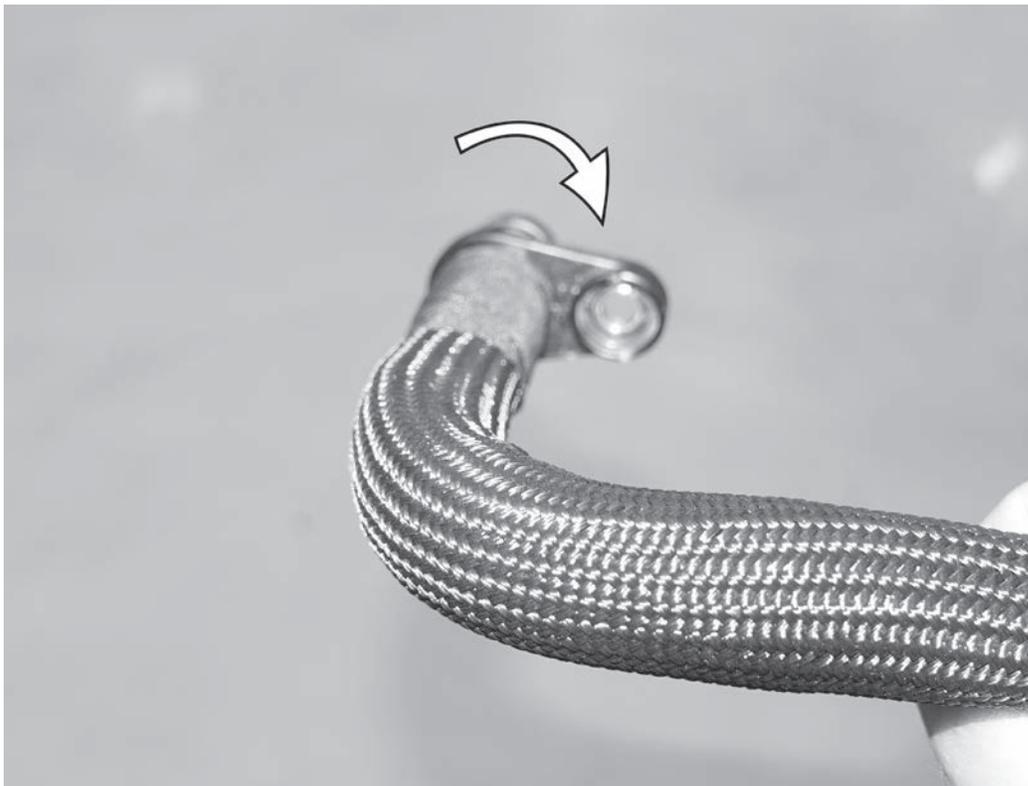
35) Rotate the end of the stock PCV hose approximately 180° by holding the hose and rotating the plastic fitting. It is not necessary to remove the fitting from the hose.
