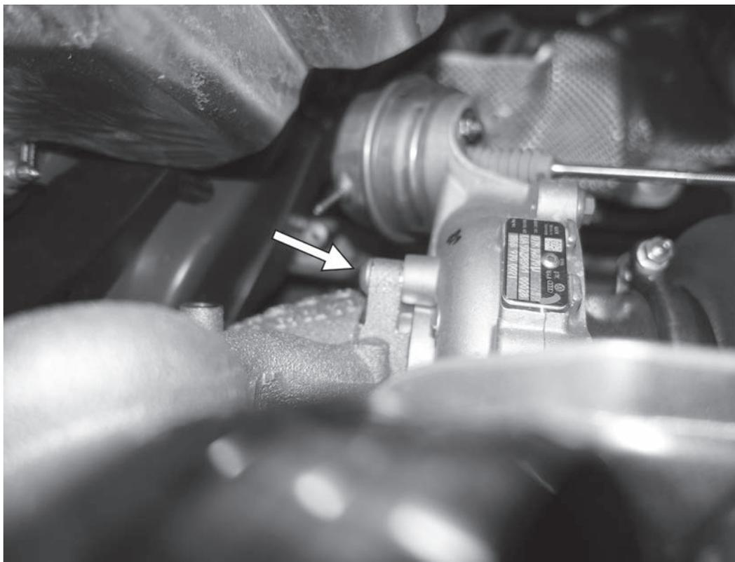
11) Locate the top T30 screw holding the upper side of the turbo inlet pipe to the compressor side of the turbocharger. Remove this screw, leaving the lower one in place.
