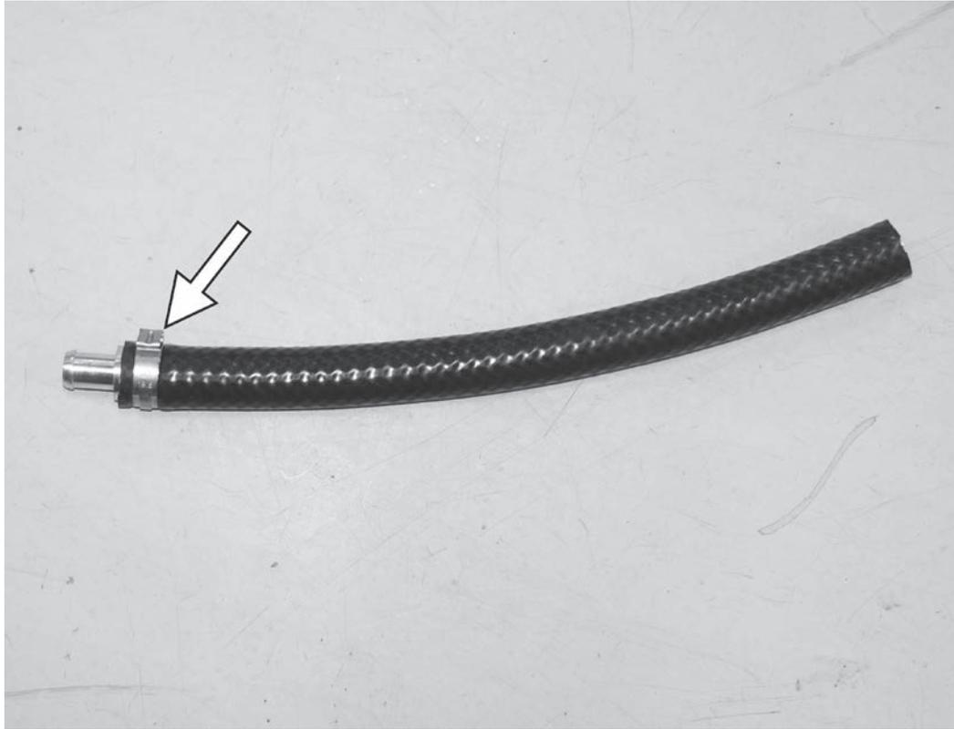
47) Make the shown assembly using the supplied parts. Crimp the barbed connection to the hose using one of the 19.8mm ear clamps.
