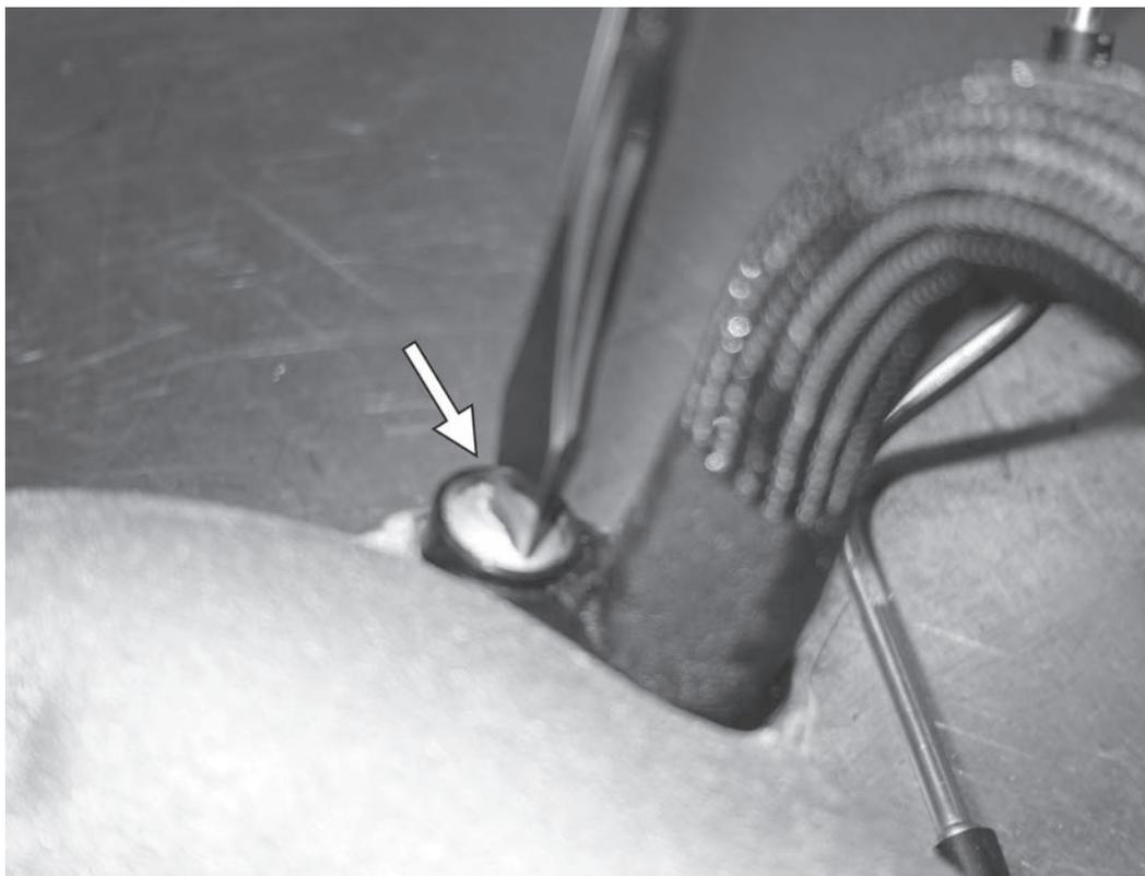
23) Using a large flathead screwdriver, push down on the previously cut slot and turn the screw to remove the PCV hose. It is easier to turn the screw if the screw is still warm from grinding the slot in it.
