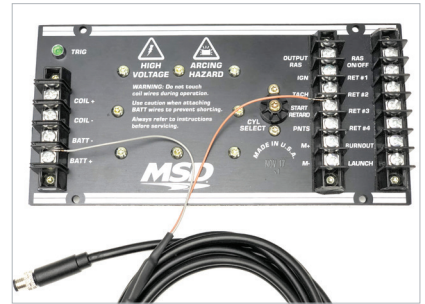
6. Route the cable to the ignition box, Brown: Ignition box Tach Output Gray: Tach Ground.
