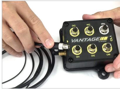
2. Connect the M8 connector to Channel 1 on the CL1 data box.
