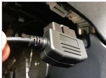
8. Vehicles utilizing Racepak's OBD2 cable, see Step 12 - OBD2, of this manual, for setup instructions.
