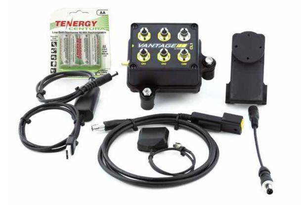
**CL1 Data Box Dimensions** 3.25" x 3.00" x 1.75" / 8.26cm x 7.62cm x 4.44 cm Weight .75lbs / 12 ounces with installed batteries Housing Injection molded plastic – water resistant **External Connectors** Four – 5 pin sensor input connectors One – 3 pin charging connector One – 6 pin CAN connector Wireless Low energy Bluetooth GPS Up to 20Hz **Power** Four – Rechargeable Ni-MH size AA batteries Inputs Eight Total – 4 Analog / 4 Digital User defined
