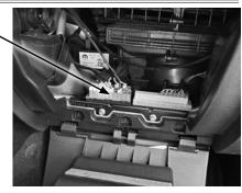
**STEP 14** - You will need to line up the glove box assist gear to its guide arm and reinsert it while lifting up on the glove box until it locks back into place.
