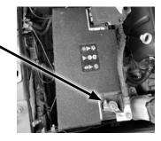
STEP 1b - The non-eTorque has a secondary battery, so you will need to remove the secondary battery cable as well. Disconnect the negative battery terminal from the battery using a 10 mm socket and a 13 mm socket, then remove the nut connecting the two negative cables to one another. Ensure that the ground cables do not contact each other during the installation process. If needed, separate them with a rag.
