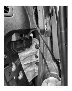
STEP 13 - After routing the CAN cable behind the glove box, connect it to ANY open spot on the green junction box. Once you have the CAN connection installed, you can put the glove box back on. Zip tie the excess cable behind the glove box in an area where it will not get pinched when the glove box is closed completely.
