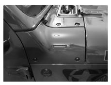
**STEP 7 (Option B)** - Use a coat hanger or fish tape to feed the CAN wire under the windshield wiper cowl. Be careful to not scratch your paint if using this option. You may want to use masking tape to prevent scratching.
