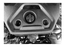
**STEP 3** - Remove the secondary plastic cover over the passenger side of the engine bay. Use a 10mm socket to remove the two mounting bolts, then pull straight up to release the cover from the rubber grommets.
