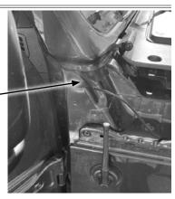
**STEP 9** - After the CAN connector is routed through the engine panel (1), you will need to route it through the door frame and through the Jeep® access panel (2) to get it into the glove compartment as images show below. Gently pry the plastic weather stripping back and route the cable behind it in a way that it won't get pinched when the door closes (3/3a).
