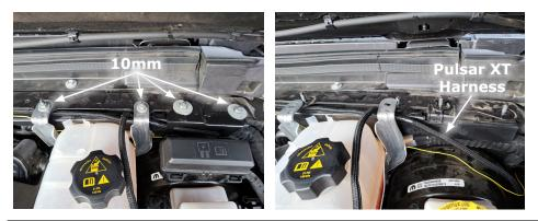
**STEP 5** - In turn, disconnect both the MAP Sensor and FRP Sensor by first pushing back on the red locking tab and then pushing in on the release tab. Connect both sensors into the Pulsar XT harness. **NOTE:** Both sensors are located between the charge air tube and battery on the passenger side of the engine
