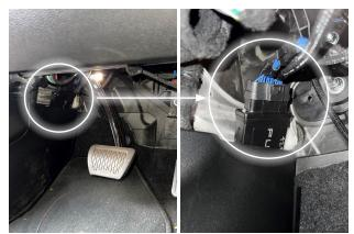
**STEP 15** - Use provided zip ties to secure excess cable away from the brake and accelerator pedals, and any hot surfaces or moving components in the cab and in the engine bay.
