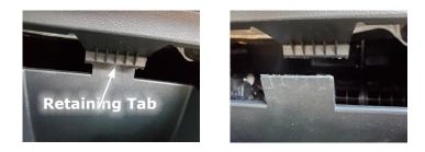
**STEP 12** - Disconnect the soft close latch on the left side of the glove box by lifting up until it clicks. Pull the soft close arm out, then the glove box will slide out.
