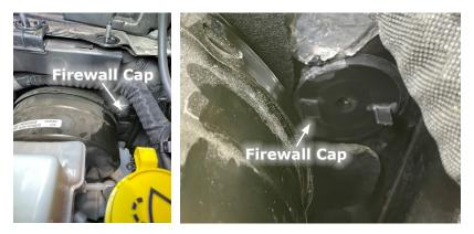
**STEP 8** - After removing the firewall cap, drill a 5/8" hole in the center of the cap, then place it back in the firewall. Route the 8-pin access link into the cab as shown on images. Then, reinstall the fusebox and nuts (from STEPS 3-4).
