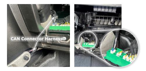
**STEP 14** - Plug in the main Pulsar XT Harness into the module and tuck the module behind the driver side kick panel. Make sure the module is pushed in enough so it sits snug.
