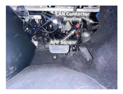
**STEP 9** - Disconnect the APP Sensor located above the accelerator pedal by sliding the locking tab away from the sensor (towards the rear of the vehicle). As the lock tab slides out, the sensor will slowly slide up and you will be able to disconnect it once the locking tab is fully released. Then, connect both ends to the Pulsar XT harness.
