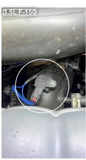
**STEP 3** - Locate the MAP sensor found on the intake manifold behind the throttle body. Disconnect the MAP sensor by sliding the locking tab then squeezing it. Connect both connectors to the Pulsar XT harness and the locking tabs.
