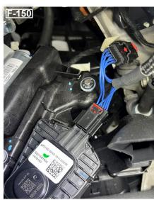
**STEP 7** - Connect the OBDII plug into the OBDII port located on the lower left side of the kick panel.
