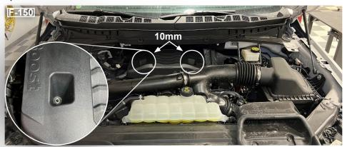
**STEP 2** - Locate the Boost Pressure Sensor connector on the charge pipe before the throttle body. Disconnect the Boost Pressure Sensor by sliding the locking tab then squeezing it. Connect both connectors to the Pulsar XT harness and lock the locking tabs.
