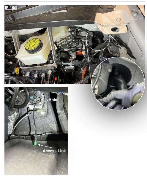
**STEP 6** - Locate the APP connector above the accelerator pedal and disconnect it by pulling up on the red lock tab and then pushing in the release tab. Connect both connectors to the Pulsar XT.
