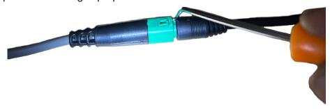
**STEP 3** - Pull the connector apart while holding the clip out.
