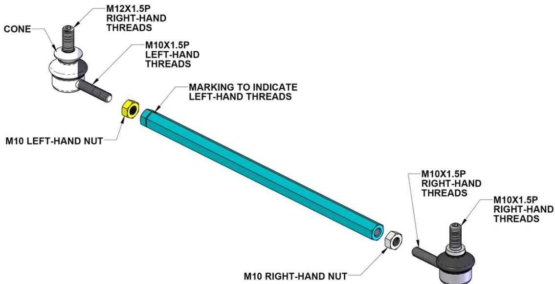
8. Adjust both links to measure 16-3/8" center-to-center, as shown below. For easy adjustment, the Dinan end links are left/right hand threaded. Failure to follow this step can result in loss of control, vehicle damage, and injury!
