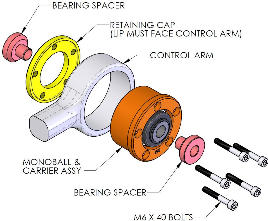
5. Install the Dinan retaining cap onto the arm (the lip must face the control arm as shown). Put a small amount of Loctite on the M6x40 bolts and torque to 95 inch-pounds to secure the retaining cap.
