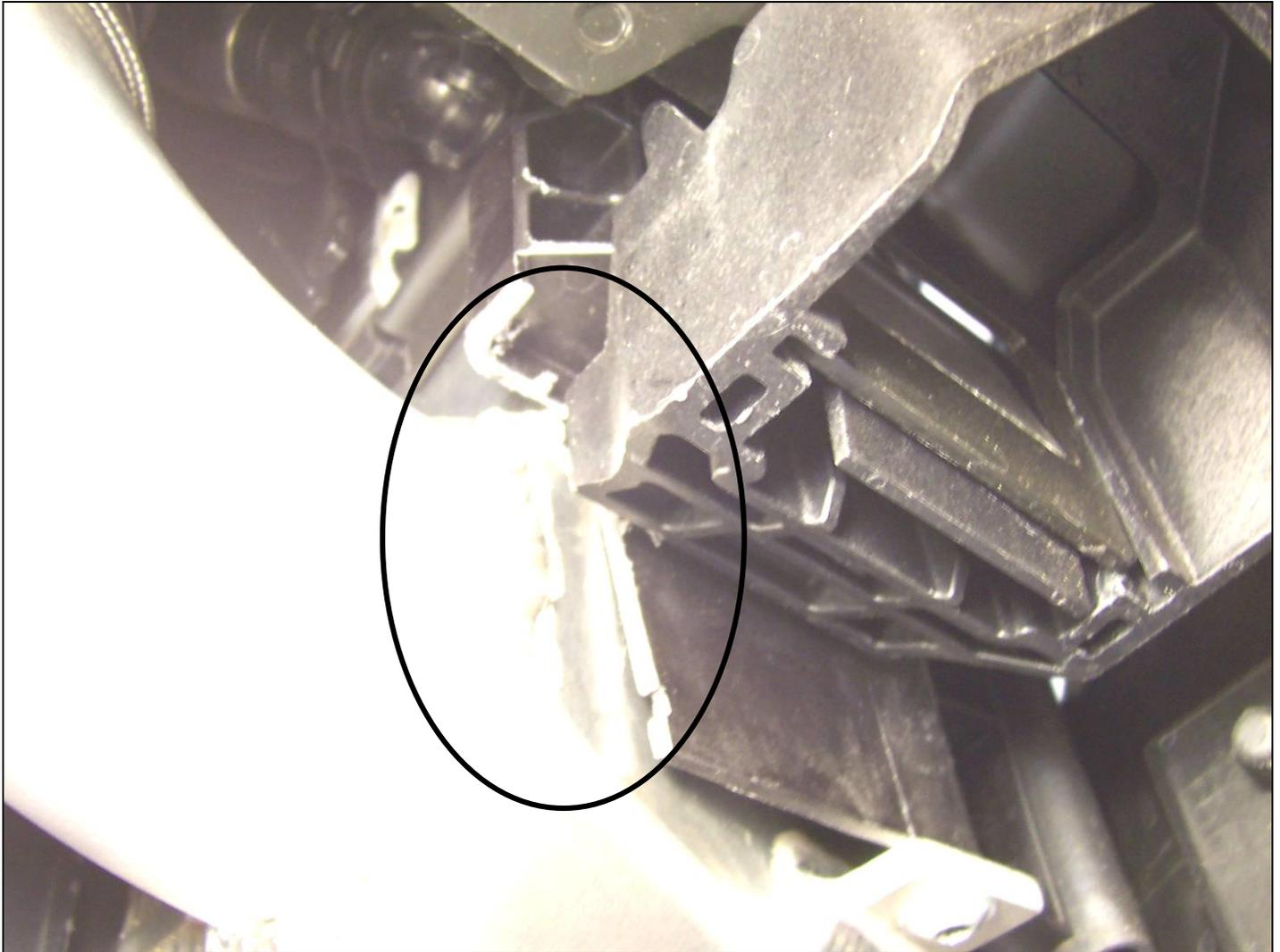
10. The cutting for most of the plastic can be done using a hacksaw and a jig saw. It is easy to cut so don't go overboard as you can always take a little more off later. Minor trimming can be done with a sanding disc or large diameter die grinder bit.
