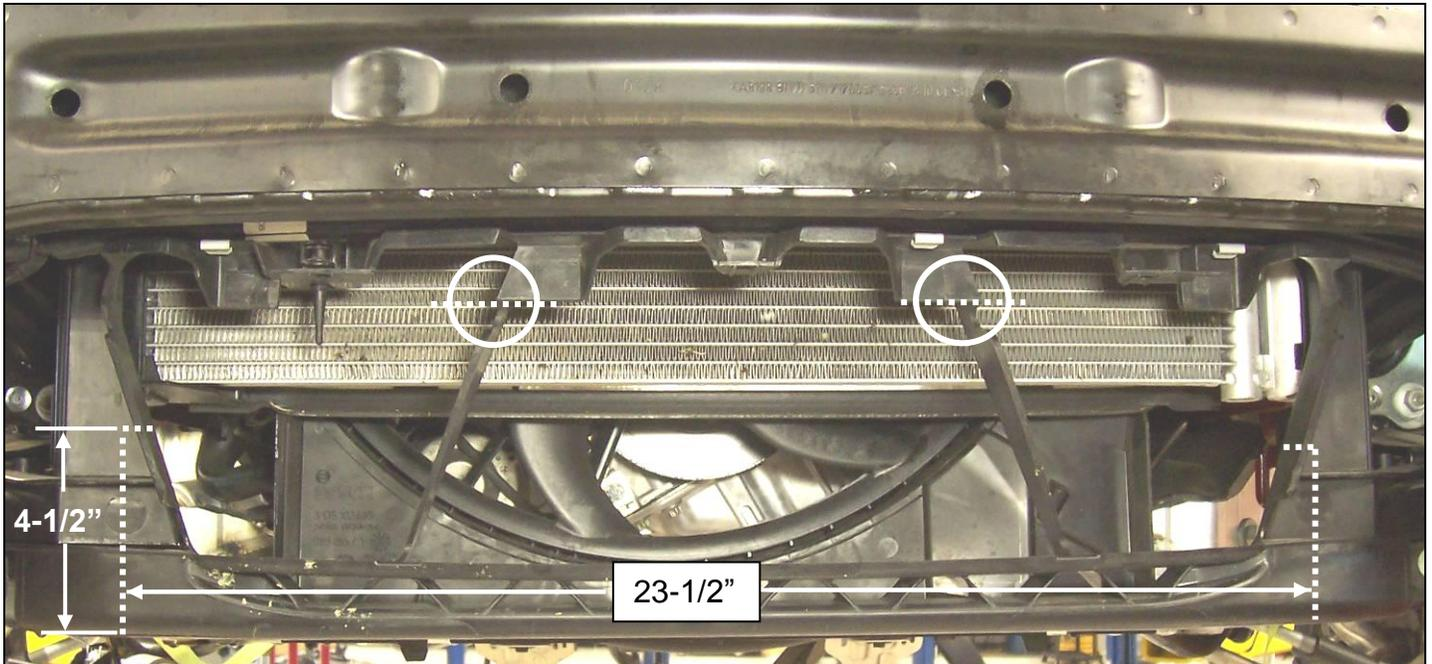
6. The photo below shows the basic installation from the front view.
