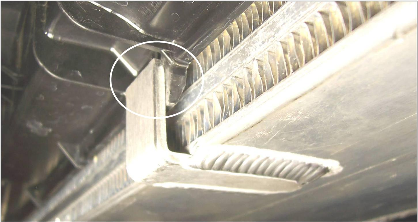
12. When you have the Intercooler opening sufficiently clearanced you will need to install the hose coupler latches from the stock intercooler onto the Dinan intercooler. Check the condition of the O-Rings on the stock hose's and replace if needed.
