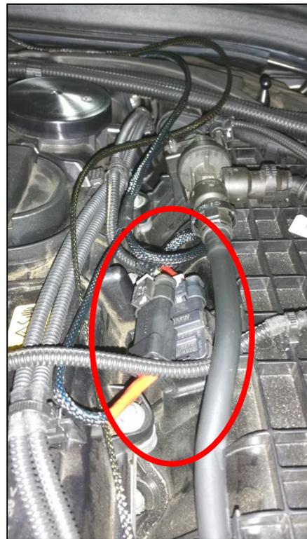
10. The SPORT module is secured using the included zip-ties. Please note -- DO NOT route the zip-tie over the harness at the SPORT module, as this could stress the internal circuit board and damage the module! Only insert a zip-tie thru the slots on the SPORT module as shown below.
