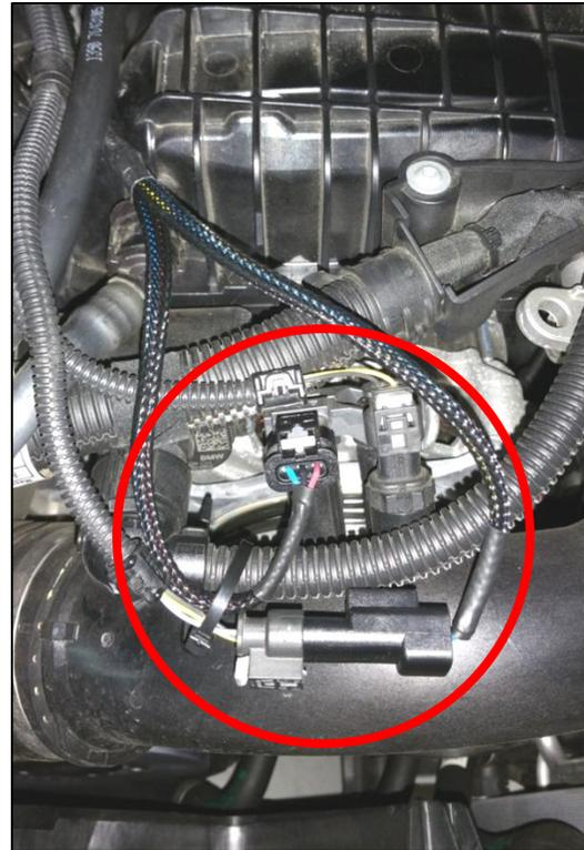
7. Referring to the photo below, locate the pressure sensor installed on the intake manifold, near the center-top of the engine.
