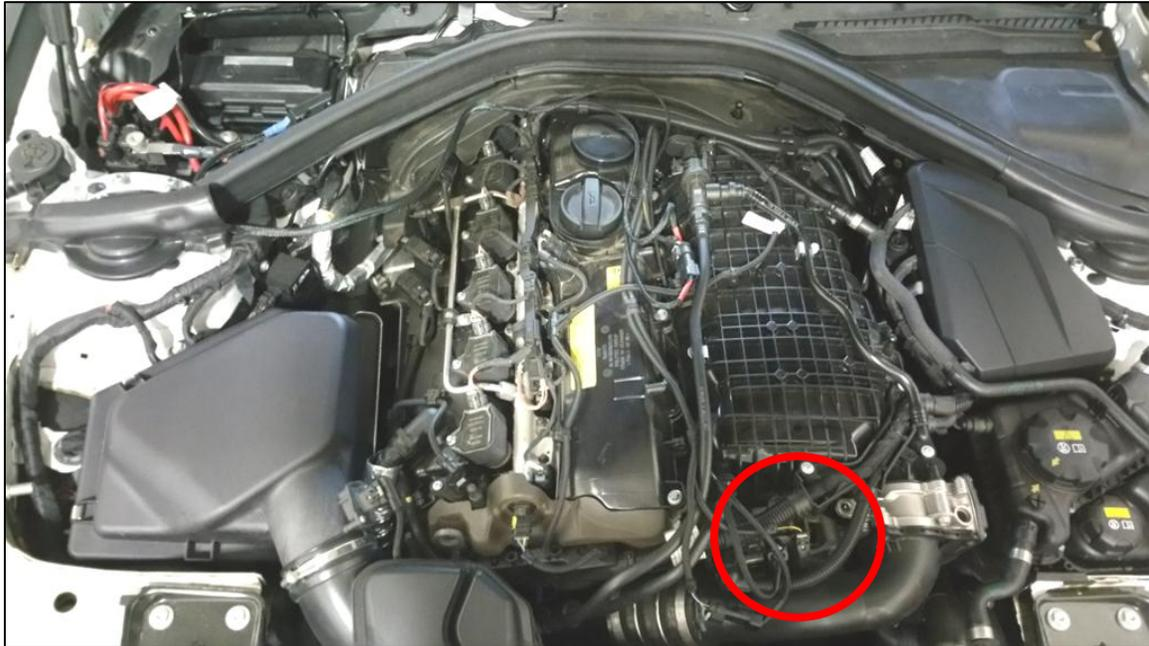
5. Disconnect the factory wiring harness from the pressure sensor. You may wish to study the locking system on the new DINANTronics SPORT connectors until you are familiar with how the two connector halves are released. Some locks will require the use of a small flat blade screwdriver to release the tang.
