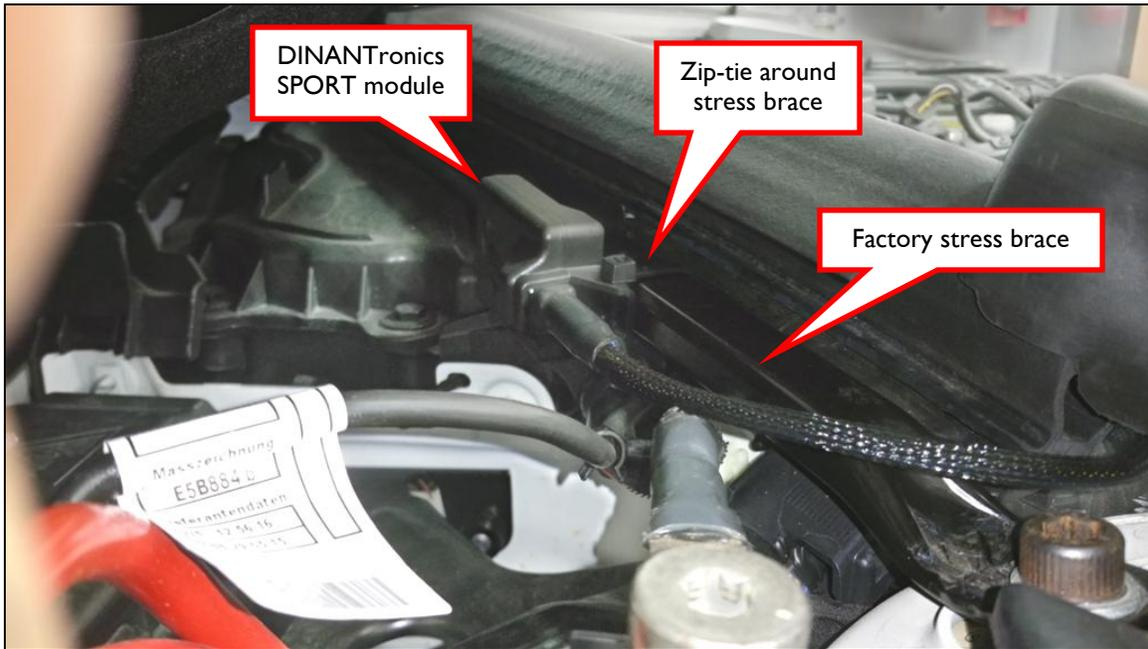
12. Route the harness as shown below, and use zip-ties to secure the wiring harness. Ensure adequate slack in the wiring harness to allow for engine movement.
