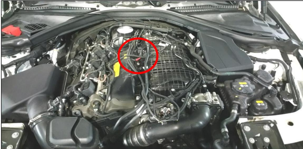
8. Disconnect the factory wiring harness from the intake manifold pressure sensor. You may wish to study the locking system on the new DINANTronics SPORT connectors until you are familiar with how the two connector halves are released. Some locks will require the use of a small flat blade screwdriver to release the tang.
