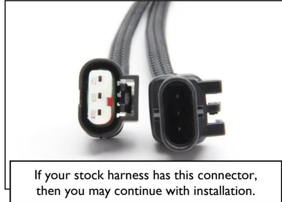
13. Like the previous sensors, install the DINANTronics harness in between the fuel rail pressure sensor and the factory wiring harness. The connectors are unique, and can only be installed one way. Make sure that the locking tangs on both connections are secure.
