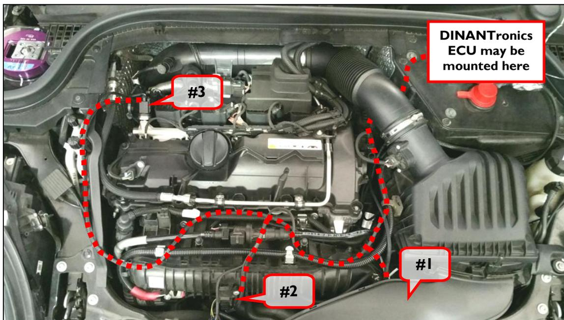
**NOTE:** There are two possible connector styles for Sensor #3. You may wish to glance at steps 11 & 12, to confirm that the connector on the Dinan harness is correct for your vehicle, before continuing with this installation.
