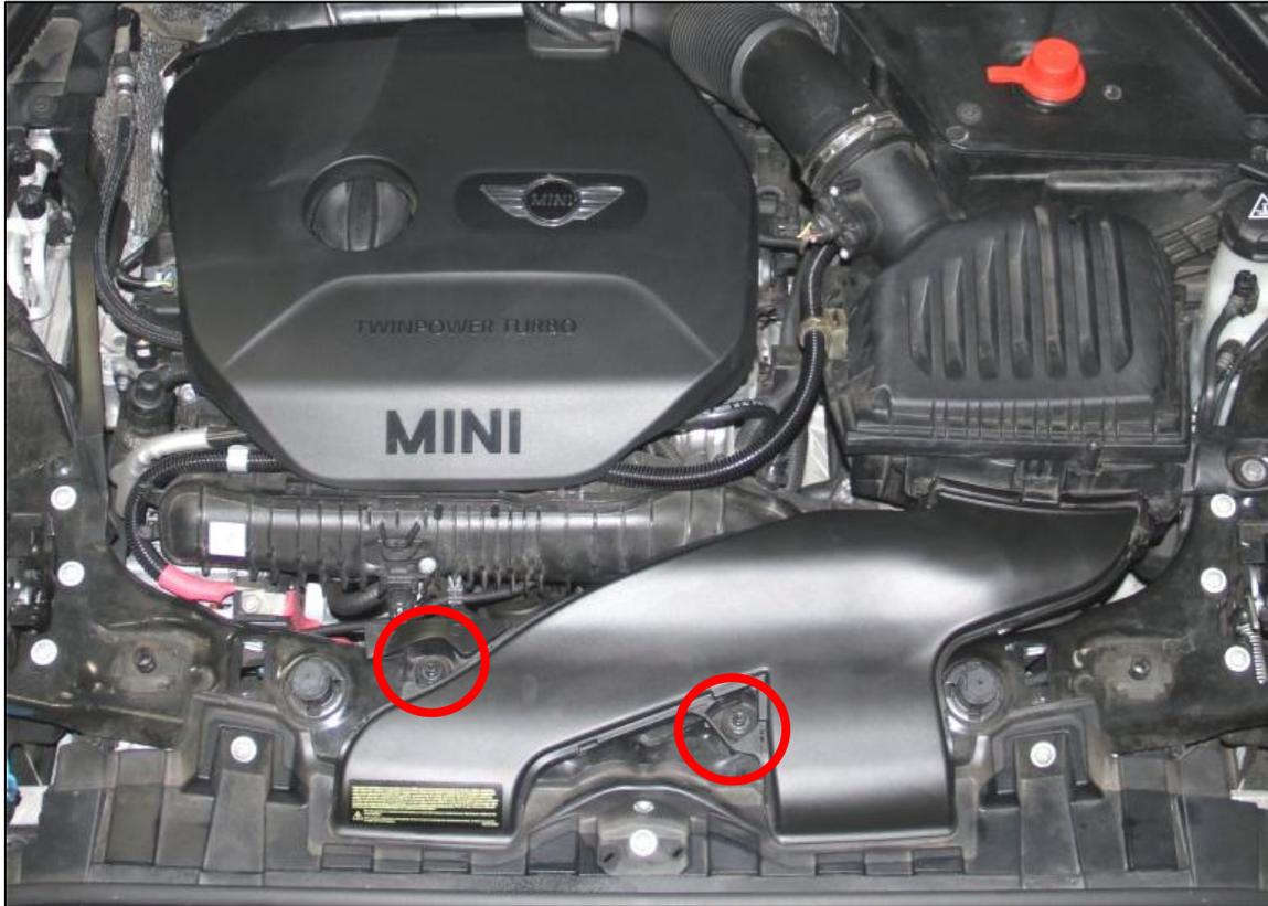
5. The charge air tube pressure sensor is shown below. It will have a connector that is identical to the ones on the DINANTronics harness.
