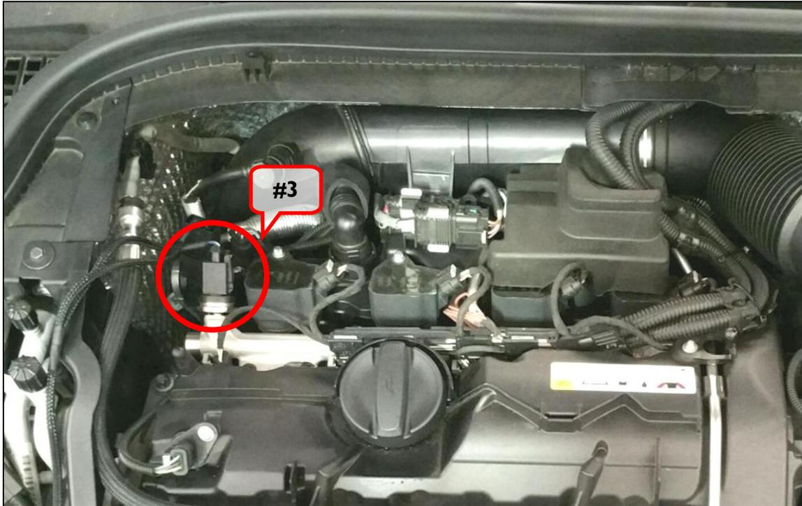
12. The fuel rail pressure sensor connection could be one of two configurations. Please examine your harness connector and compare it to the photos below. One style is a D-shape, while the other style is an oval-shape. If you do not have the correct harness for your vehicle, please contact Dinan for an exchange -- do not continue with installation
