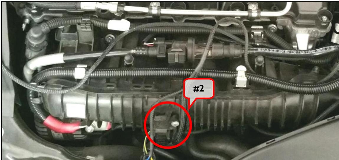
10. Like the previous sensor, install the DINANTronics harness in between the manifold pressure sensor and the factory wiring harness. The connectors are unique, and can only be installed one way. Make sure that the locking tangs on both connections are secure.
